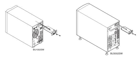
(2) After changing the settings, carefully reinsert the contact signal card and securely tighten the 2 screws.
